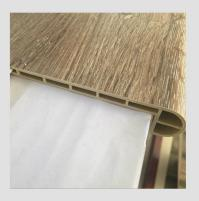
Stair nose molding is used in conjunction with floor installation to finish off the step or stairwell where the floor stops. Stair nose molding is about 5 inches wide, with a rounded bullnose edge that extends down to cover the edge of the step
